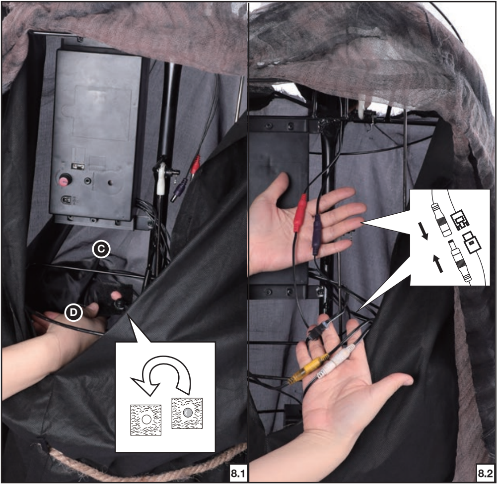
STEP 8 Secure Sensor to the sensor hole on the (C) Costume using the hook and loop closure as shown in Figure 8.1. And connect all cables from the Function Control Box to their corresponding cables by color as shown in Figure 8.2.
